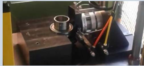
*Spin testing under load ensures against defects to each bearing's rollers or raceway.*
